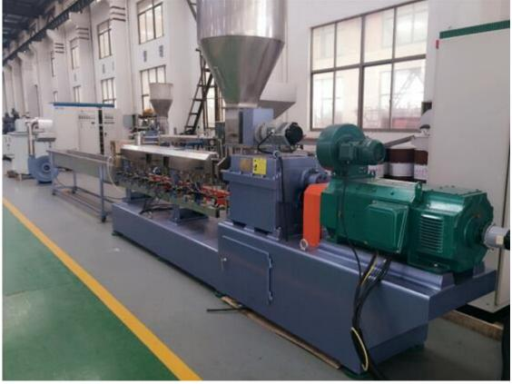
A TSK-65 line ready for pre-shipment test. (The picture is only for reference)
