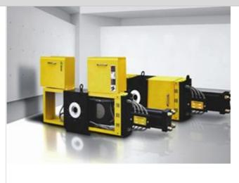
The strand die photo is only for reference Motor power: 2.2kW (3 hp) Material: 38CRMoAl Number of strands: 13-15
